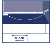
Step 3: Use leftover flooring from first row as starter for second row. There must be at least 8" (20cm) between flooring end joints on adjacent rows. FOR TILE INSTALLATIONS: The distance between end joints should be equal to 12"(30cm) for proper appearance.
