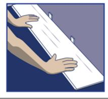
Step 1: Begin installation working from left to right. Insert spacers at ends and edges where flooring meet wall. Use 1/4"spacer's along walls to maintain proper expansion space.
