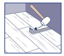
Step 9: Use rubber mallet and pull bar to lock long edges of flooring on final row.
