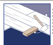
Step 7: Tap end of flooring with rubber mallet and tapping block to lock ends of flooring together. Remove bridge and continue towards wall until installing the final flooring in the row.
