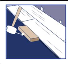
Step 5: IMPORTANT! Use rubber mallet and tapping block to tap long edge of plank to ensure a tight fit. ANY GAPPING CAN COMPROMISE THE LOCKING SYSTEM!
