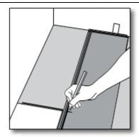
Place the final plank face down with the short side (without the locking strip) towards the wall. The remaining expansion space should be a minimum 1/4" from the wall. Draw a pencil line where the plank is to be cut.
