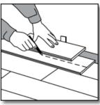
Measure and cut the last row to fit, remember to allow for a minimum of 1/4" expansion space from the wall. Use a full width scrap plank to mark your cutting on the last row.
