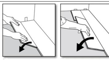
Place the plank at an angll against the plank in the previous row, press the edge forward against the previous row and fold down at the same time.
