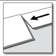
In the first row, place the second plank tight against the short end of the first plank.
