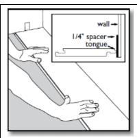
Begin the installation in the left-hand corner. Place the plank a minimum of 1/4" from the left wall.
