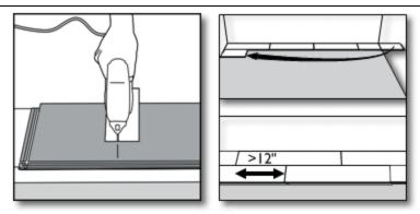
Place the plank face down on the work surface and cut to size with a power saw. If you are using a hand saw, use a fine-toothed blade, and cut the planks face up. The score/snap method (using a square or straightedge) requires the pad be cut from the back side using a utility blade (either before or after the score/snap).
