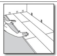
The distance to the walls can be adjusted when three rows have been completed. Remember to place the flooring a minimum of 1/4" from all walls or other vertical obstructions such as cabinets, pipes, or columns.
