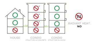
Installation on the ground floor and upstairs only. Do not install in the basement or below grade.
