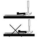
Repeat the process approximately every 12" (30cm) until the entire long edge of the plank has clicked in with the next plank.
